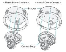
2 Connect the cable through the cable hole and screw the safety wire to the bracket to prevent the bracket from falling on to the floor.
