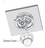
5 Assemble the bracket lid to the bracket.
